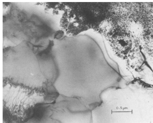
Figure 14 Interface (indicated by arrows) of powder and Ni electroplating, as seen in thin foil. Possible fine precipitates at powder surface are largely obscured by small grains of Ni plating.
